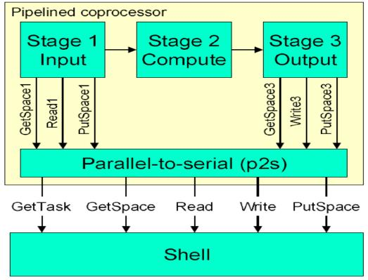
Fig.4. A model Pipelined Co-Processor
